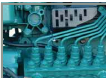
Well balanced engine block 6 in line cylinders
